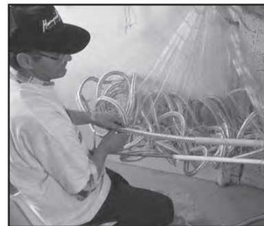
6. The rope is now drawn through the pipe and the selvage is pulled onto it from the pipe at the required interval. The hanging ratio is 50%. When the rope is drawn through the pipe, the knotted selvage meshes tightens to it.
