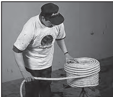
1. The coil is placed on a turntable before it is unwound.
