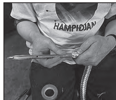
7. Braided float ropes are easy to join. Firstly, the floats are removed along a 50 cm section. Each end is cut to a taper and covered with tape. A braiding needle is used to pierce the rope and one rope end is stuck into the middle of the other.
