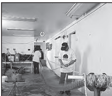
4. Once the net has been threaded onto the plastic pipe, the ends are fixed. A rope of 10-12 mm is pulled through the end meshes later to be fastened to the lead rope and float rope.
