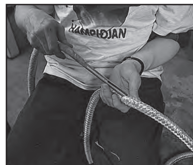
8. Repeat for the other end and finally staple or sew down.
